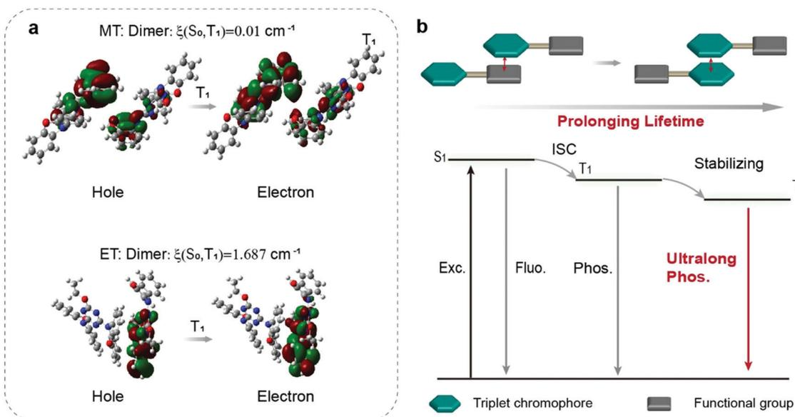
**Fig. 4** Proposed mechanism for ultra-long phosphorescence (a). Natural transition orbitals (NTOs) of T<sub>1</sub> states for the MT and ET dimer. (b) The mechanism of the different emission behaviours in the compound.
