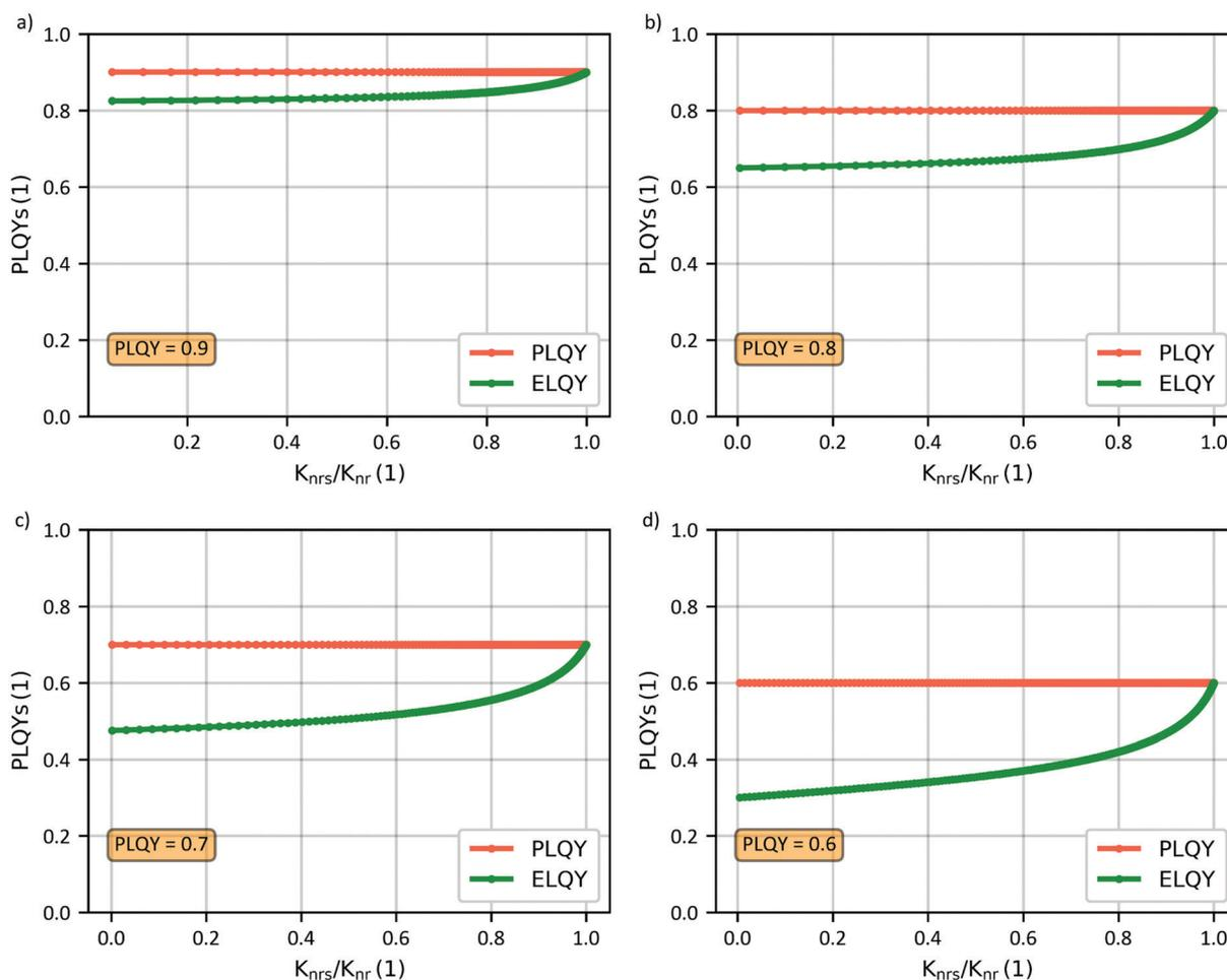
**Fig. 2** For a fixed PLQY of 0.9 (a), 0.8 (b), 0.7 (c), 0.6 (d) the ELQY is calculated for all possible couples  $k_{\text{nrs}}-k_{\text{nrt}}$  which are solutions of eqn (1). In this calculation the other rates have been supposed known ( $k_f = 10^7 \text{ s}^{-1}$ ,  $k_{\text{isc}} = 10^7 \text{ s}^{-1}$  and  $k_{\text{risc}} = 10^6 \text{ s}^{-1}$ ).
