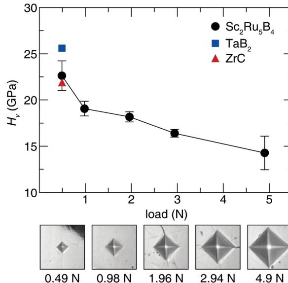
Fig. 2 Vickers microindentation ( $H_V$ ) measurements of  $\text{Sc}_2\text{Ru}_5\text{B}_4$  from low (0.49 N) to high (4.9 N) load and  $\text{TaB}_2$  and  $\text{ZrC}$  at low (0.49 N) load. Error bars correspond to the average error of multiple independent measurements. Representative indentations from each applied load are shown below the plot.
