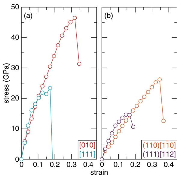
Fig. 7 Calculated stress-strain curves for  $\text{Sc}_2\text{Ru}_5\text{B}_4$  (a) Stress-strain curves for various crystallographic directions under applied tension. (b) Stress-strain curves for the hardest and softest shear systems.
