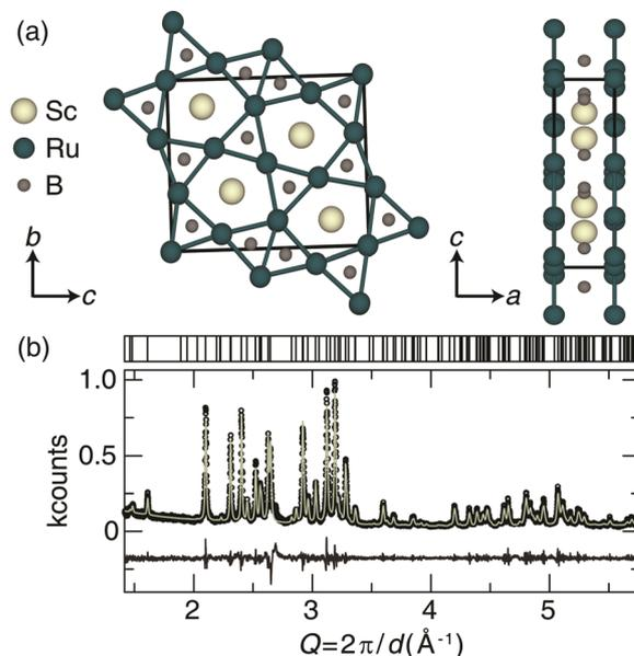
Fig. 1 (a) Single-crystal structure of orthorhombic  $\text{Sc}_2\text{Ru}_5\text{B}_4$ , where scandium is cream, ruthenium is teal, and boron is dark gray shown along the  $a$ -direction (left) and along the  $b$ -direction (right). (b) Le Bail refinement of  $\text{Sc}_2\text{Ru}_5\text{B}_4$ . Black circles represent the measured data, the refinement fit is in cream and the black line represents the difference.
