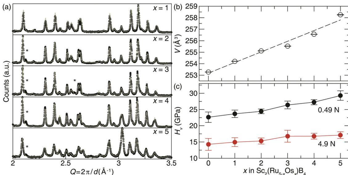
Fig. 3 (a) Powder X-ray diffractograms of the solid solution  $\text{Sc}_2(\text{Ru}_{5-x}\text{Os}_x)\text{B}_4$  ( $x = 1-5$ ). (b) The refined volume determined from Le Bail refinements as a function of  $x$  follows Vegard's law. (c) Vickers microindentation ( $H_V$ ) measurements of  $\text{Sc}_2(\text{Ru}_{5-x}\text{Os}_x)\text{B}_4$  at low load (0.49 N) and high load (4.9 N).
