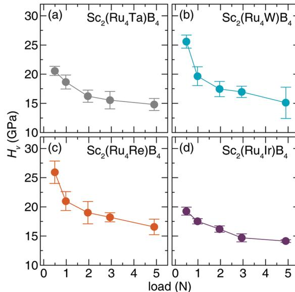
Fig. 6 Vickers microindentation measurements of (a)  $\text{Sc}_2(\text{Ru}_4\text{Ta})\text{B}_4$  (b)  $\text{Sc}_2(\text{Ru}_4\text{W})\text{B}_4$ . (c)  $\text{Sc}_2(\text{Ru}_4\text{Re})\text{B}_4$  (d)  $\text{Sc}_2(\text{Ru}_4\text{Ir})\text{B}_4$  from low (0.49 N) load to high load (4.9 N).
