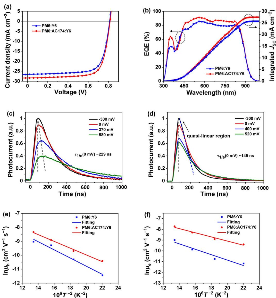
Fig. 2 (a)  $J$ - $V$  curves and (b) EQE and integrated  $J_{\text{SC}}$  curves of optimized PM6:Y6 and PM6:AC174:Y6 devices. TPC curves of (c) PM6:Y6 and (d) PM6:AC174:Y6 devices at varied external bias voltages. Temperature dependence of hole mobility (e) and electron mobility (f) of PM6:Y6 and PM6:AC174:Y6 films in a  $\ln \mu$  vs.  $T^{-2}$  representation for quantitative analysis of the energy disorder.
