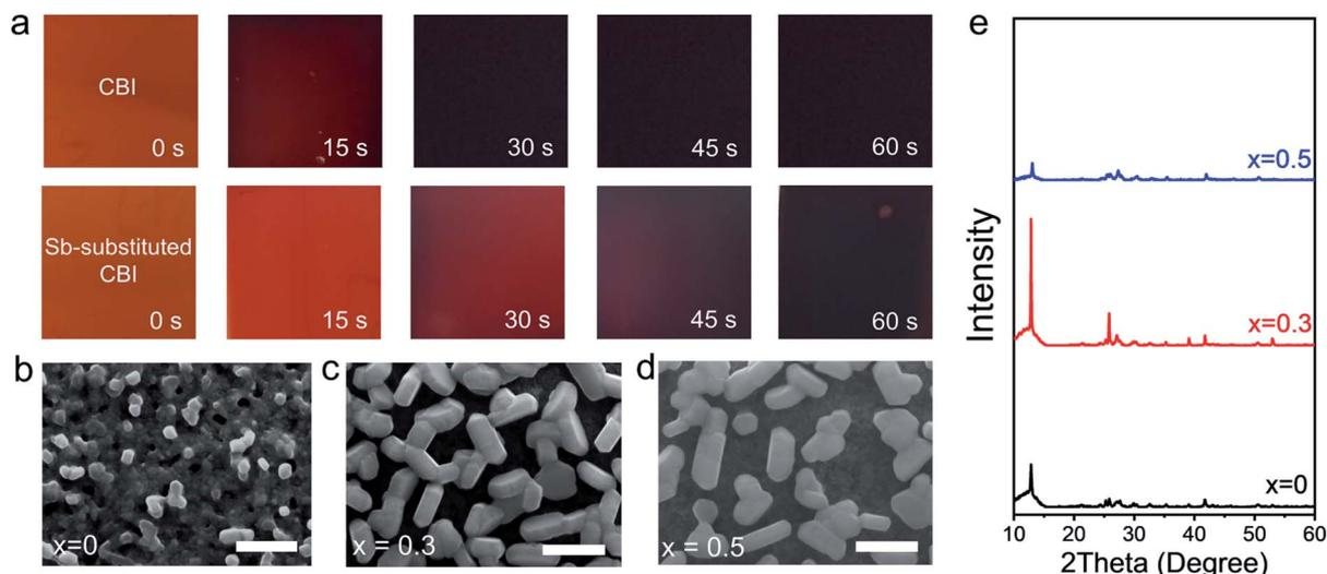
Fig. 1 (a) Photographs of  $\text{CsBi}_3\text{I}_{10}$  (CBI) and  $\text{Cs}(\text{Bi}_{0.7}\text{Sb}_{0.3})_3\text{I}_{10}$  (CBSI-3) films with different thermal annealing duration. SEM images of (b) CBI, (c) CBSI-3, and (d) CBSI-5 films, the scale bar corresponds to 500 nm. (e) XRD patterns of CBI ( $x = 0$ ), CBSI-3 ( $x = 0.3$ ), and CBSI-5 ( $x = 0.5$ ) films. (All films illustrated here are synthesized from DMF/DMSO mixed solvent with the volume ratio of 9 : 1).
