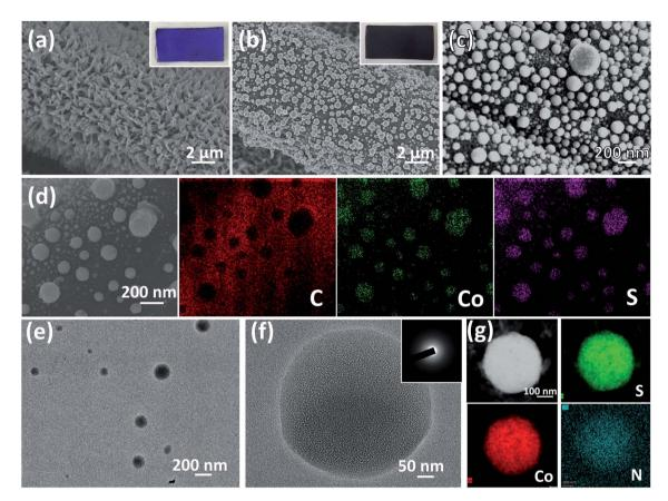
Fig. 1 SEM images of Co-MOF/CC (a) and CoS<sub>x</sub>/CC-L (b and c). Insets are the corresponding photographs. (d) Corresponding EDS mapping of the C element, Co element and S element for  $CoS_x/CC-L$ . TEM (e) and HRTEM (f) images of  $CoS_x/CC-L$ . The inset in (f) is the SAED pattern of CoS<sub>x</sub>/CC-L. (g) Elemental mapping of CoS<sub>x</sub> nanospheres.
