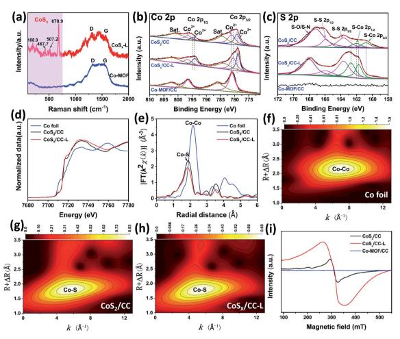
Fig. 2 (a) Raman spectra and high-resolution XPS spectra of the Co 2p (b), S 2p (c) for Co-MOF/CC,  $CoS_x/CC-L$  and  $CoS_2/CC$ . (d) Normalized Co K-edge XANES spectra and (e) Fourier transform of  $k^2$ -weighted Co EXAFS spectra of Co foil, CoS<sub>x</sub>/CC-L and CoS<sub>2</sub>/CC. (f-h) WT-EXAFS spectra of the Co foil, CoS<sub>2</sub>/CC and CoS<sub>x</sub>/CC-L. (i) EPR spectra of Co-MOF/CC, CoS<sub>x</sub>/CC-L and CoS<sub>2</sub>/CC.
