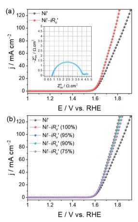
Fig. 4 (a) OER LSVs of the Ni foam electrode with and without  $iR_u$  drop correction. Inset of (a) is the normalized Nyquist plot of the same. (b) The same LSV with different percentages of  $iR_u$  drop correction.
