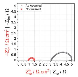
Fig. 2 Nyquist plot of the SS electrode  $(0.3 \text{ cm}^2)$  acquired at 1.674 V vs. RHE from 100 kHz to 0.1 Hz with (red) and without (black) geometrical area normalization.
