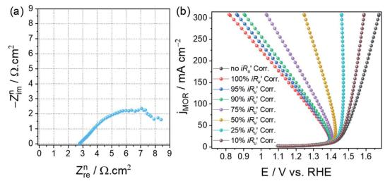
Fig. 5 (a) Normalized Nyquist plot of anodized Cu foam containing Ni impurities. (b) MOR LSVs of the same with different percentages of  $iR_u$  drop correction. Reproduced and modified from our earlier work (ref. 23) (Copyright 2021, American Chemical Society).
