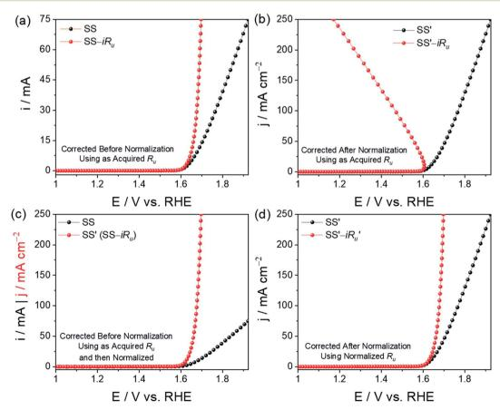
Fig. 3 (a-d) LSVs of the SS electrode with (red) and without (black)  $iR_{11}$  drop correction following different practices of  $iR_{11}$  drop correction.
