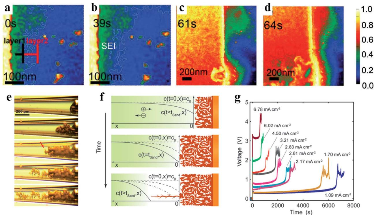
Fig. 2 Formation of SEIs and lithium dendrites. (a–d) Time sequential high-angle annular dark-field STEM (HAADF-STEM) images of SEIs. Reproduced with permission.<sup>46</sup> Copyright 2019, Wiley-VCH. (e) *In situ* optical photograph of lithium growth. (f) Theoretical interpretation of lithium deposition during concentration polarization. (g) Voltage responses under various current densities. Reproduced with permission.<sup>48</sup> Copyright 2016, The Royal Society of Chemistry.
