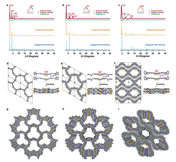
Fig. 2 (a), (b) and (c) Experimental and simulated PXRD patterns of PTz-TPB-COF, PTz-BTA-COF, and PTz-Py-COF, respectively. (d), (e) and (f) Top and side views of the unit cells in eclipsed stacking mode. The dihedral angles of the two benzene rings in phenothiazine moieties and the  $\pi$ - $\pi$  distance of the two layers are also provided. Color code: H, white; C, gray; N; blue; S, yellow. (g), (h) and (i) Graphic views of eclipsed AA stacking structures of the three COFs
