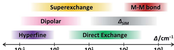
Fig. 11 The schematic representation of the energy ranges that the discussed magnetic couplings usually affect, along with the single-ion \Delta_{\text{SIM}} , in a lanthanide-based SMM.
