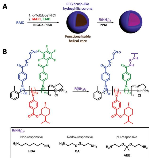
**Scheme 1** (A) Overview of the NiCCo-PISA of block copolymer micelles and post-polymerisation modification (PPM). (B) Detailed PPM procedure for the development of cross-linked and stimuli-responsive nanomaterials.
