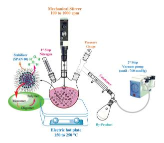
Fig. 12 Synthesis of PBS via suspension polymerization.
