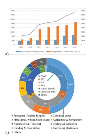
Fig. 6 Global production of bioplastics in 2021 by (a) volume (in kilo tonnes) (b) polymer type (bio-degradable) and segment (non-biodegradable and biodegradable).
