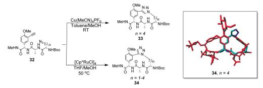
Scheme 6 Synthesis of 1.4- and 1.5-triazole linked DE-ring mimics 33 (n = 4) and 34 (n = 1-4) from linear precursor 32 using Cu-catalysed and Ru-catalysed azide-alkyne cycloadditions. Energy minimisation acquired with AMBER99 forcefield shows 34 (n = 4) in blue superimposed onto balhimycin shown in red.
