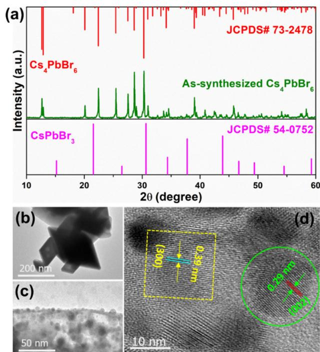
Fig. 2 (a) Powder XRD pattern of the Cs<sub>4</sub>PbBr<sub>6</sub> microcrystals (MCs), (b and c) TEM and (d) HR-TEM images of the Cs<sub>4</sub>PbBr<sub>6</sub> MCs embedded with CsPbBr<sub>3</sub> nanocrystals (NCs).
