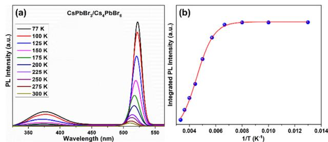
**Fig. 7** (a) Temperature-dependent photoluminescence spectra of dual-phase CsPbBr<sub>3</sub>/Cs<sub>4</sub>PbBr<sub>6</sub> MCs measured in the temperature range of 77–300 K under  $\lambda_{\text{exci}} = 315$  nm, and (b) integrated photoluminescence intensity of the green peak as a function of temperature.
