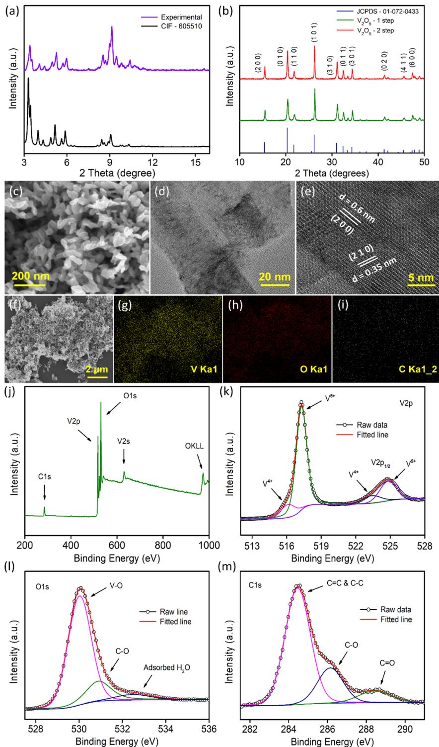
**Fig. 1** (a) XRD pattern of the activated V-MOF (purple) and the reported data CIF – 605510; (b) XRD data of  $V_2O_5$  samples along with JCPDS card (01-072-0433) data; (c) FESEM image, (d) TEM image, (e) HRTEM image of the  $V_2O_5$ -1 sample and (f–i) EDX data for its elemental mapping, (j) XPS survey spectrum of the  $V_2O_5$ -1 sample and deconvoluted XPS spectra of (k) V 2p, (l) O 1s and (m) C 1s levels.
