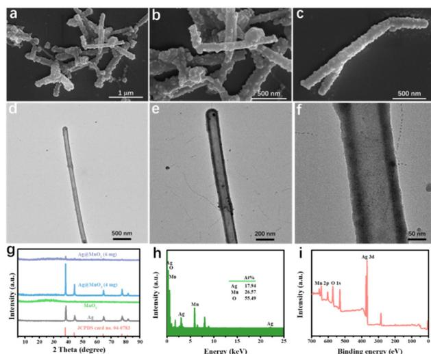
**Fig. 1** Characterizations of Ag@MnO<sub>2</sub> (a–c) FESEM images; (d–f) low-magnification TEM images; (g) XRD patterns; (h) EDX spectrum; (i) XPS survey spectrum.
