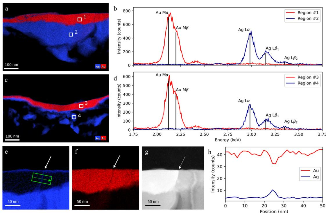
**Fig. 6** STEM-EDX analysis of a sample taken in an adjacent region to the *Mary* sample: (a and b) EDX elemental maps for Au and Ag, and EDX spectra of area 1 and 2; (c and d) EDX elemental maps for Au and Ag, and EDX spectra of area 3 and 4; (e–g) EDX Au and Ag maps and high-angle annular dark-field (HAADF) image of a gold grain boundary filled with silver atoms; (h) EDX line profile across a gold layer grain boundary (along the green arrow). Sub-panels (e–h) reproduced from ref. 38.
