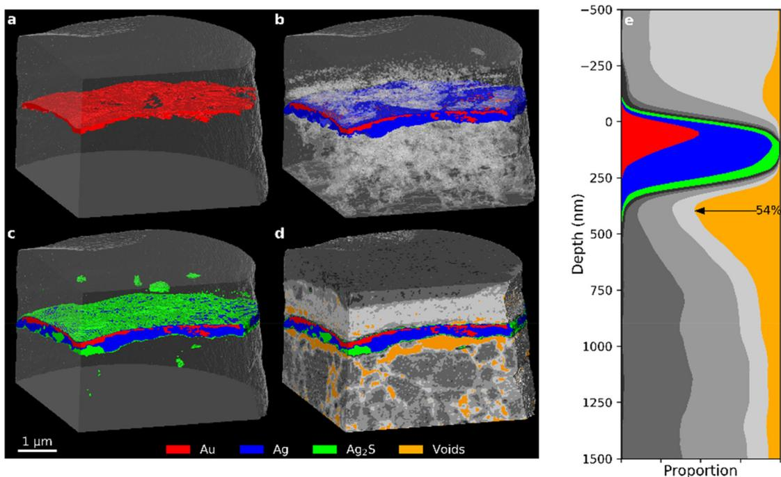
**Fig. 5** PXCT 3D images of the *Mary* sample showing the addition of (a) Au, (b) Ag (with transparent voids), (c) “silver corrosion products”, and (d) other segments (see Fig. 7 for segmentation details). (e) Stack plot of the depth profile of the sample, aligned to the main layer of the Au segment.
