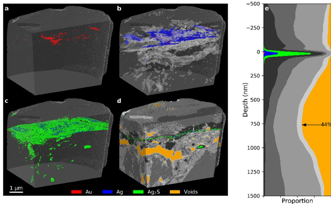
**Fig. 11** (a–d) PXCT 3D images for different components (see Fig. 7 for segmentation details) inside the Sedrun *Bishop* sample. (e) Stack plot of the depth profile of the sample, aligned to the upper surface of the metal layer.
