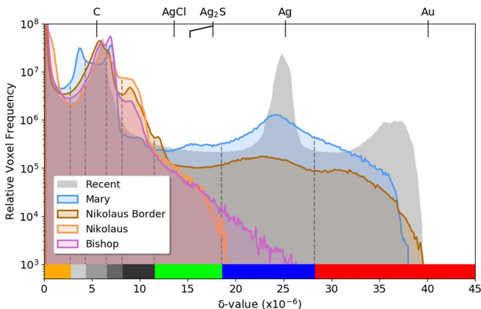
**Fig. 7** Comparison between the delta value histograms of the samples *Nikolaus Border*, *Nikolaus*, *Bishop* and *Mary*, together with the *Recent* histogram for a comparison to modern Zwischgold. The data has been median-filtered in order to decrease peak widths and the histograms have been scaled to normalise against different sample sizes. The colour bar along the lower edge indicates the segmentation for the PXCT 3D model presentations shown in other figures.
