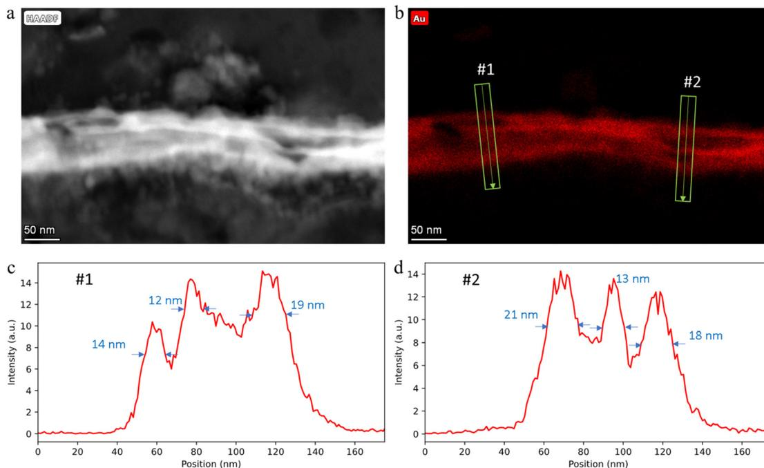
**Fig. 12** STEM-EDX analysis of a sample taken in an adjacent region to the *Bishop* sample: (a) high-angle annular dark-field (HAADF) image and (b) EDX Au map of a Zwischgold leaf cross-section; (c and d) EDX line profile across the leaf along the green arrows in (b).
