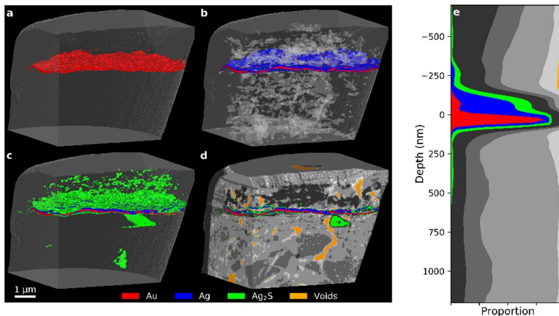
**Fig. 8** (a–d) PXCT 3D images for different components (see Fig. 7 for segmentation details) inside the *Nikolaus Border* sample. (e) Stack plot of the depth profile of the sample, aligned to the main gold layer.
