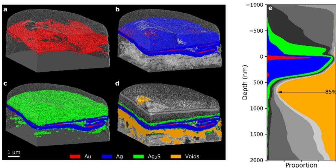
Fig. 4 PXCT 3D images of the 35-year old *Zwischgold* sample showing the addition of (a) Au, (b) Ag (with transparent voids), (c) “silver corrosion products”, and (d) other segments (see Fig. 3 for segmentation details). (e) Stack plot of the depth profile of the single-layered section of the sample, aligned to the main layer of the Au segment.
