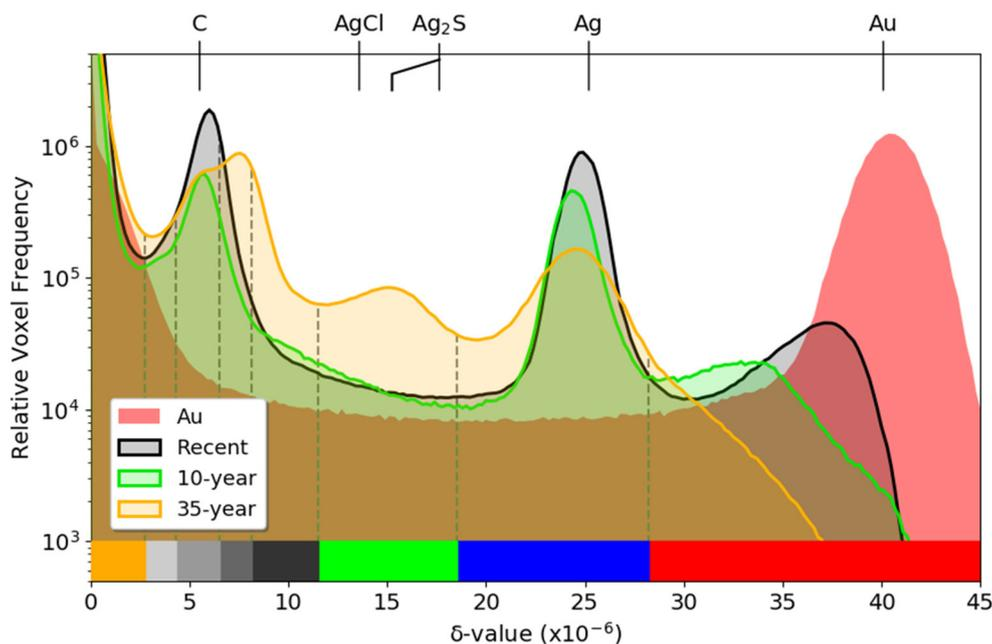
**Fig. 3** Comparison between the PXCT  $\delta$ -value histograms of the *Recent*, *10-year*, and *35-year* samples and a pure gold reference. The histograms have been scaled to match the average number of total voxels with a  $\delta$ -value above  $3 \times 10^{-6}$  in order to normalise against different sample sizes. The colour bar along the lower edge indicates the segmentation for the PXCT tomogram presentations shown in other figures.
