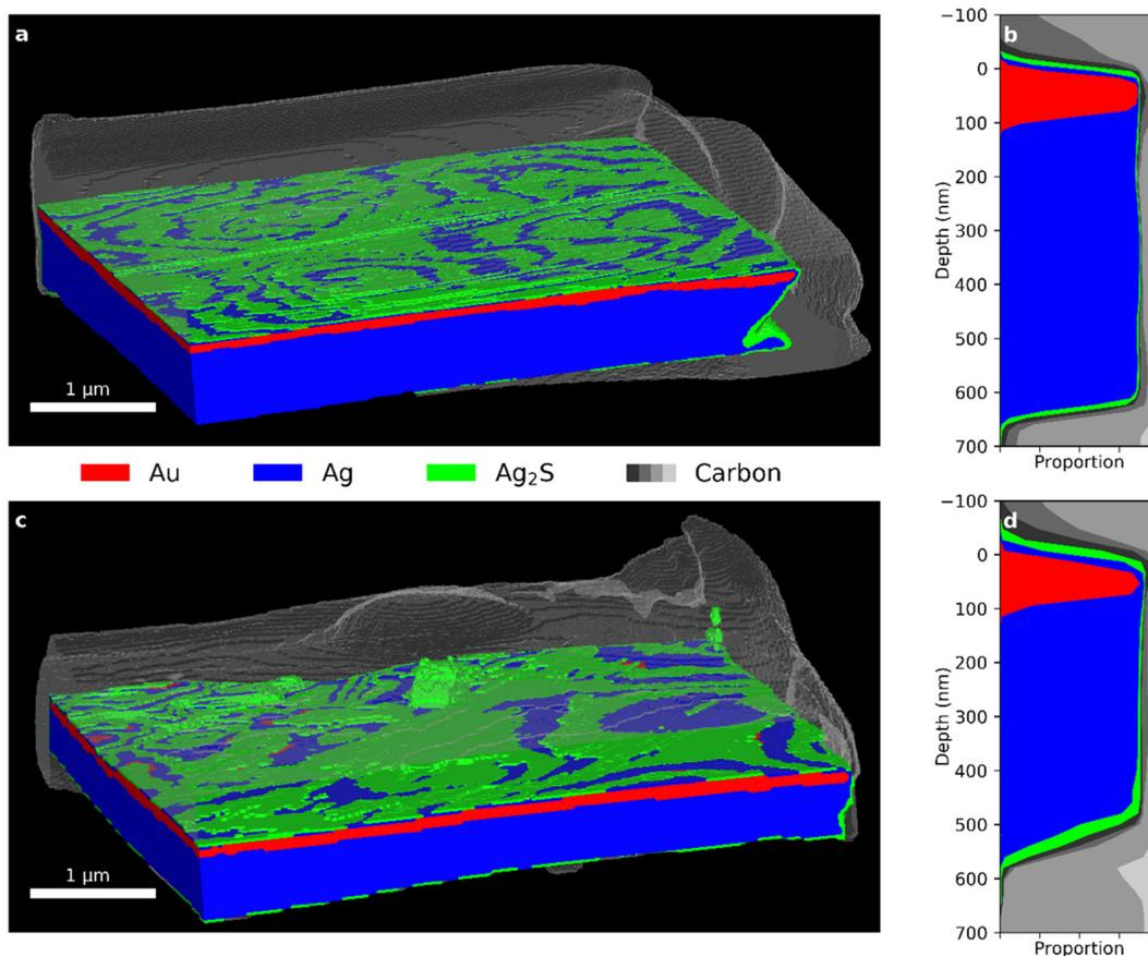
**Fig. 2** (a) Segmented PXCT 3D view and (b) depth profile of the *Recent* sample. (c) Segmented PXCT 3D view and (d) stack plot of the depth profile of the *10-year* sample. (See Fig. 3 for further segmentation details.).
