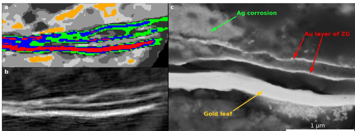
**Fig. 9** (a) A segmented and (b) raw PXCT tomogram slice for *Nicolaus Border*; (c) SEM image of a microtomed cross-section of the "Nicolaus Border" sample labelled with observations from EDX analysis. Scale bar applies to all images.
