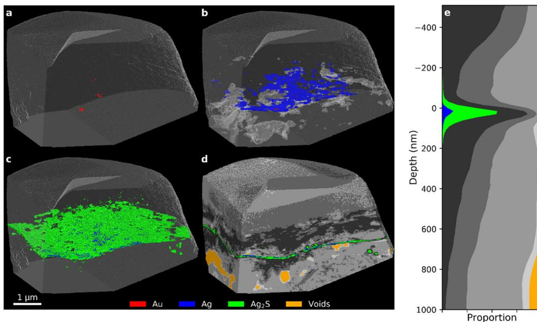
**Fig. 10** (a–d) PXCT 3D images for different components (see Fig. 7 for segmentation details) inside the Sedrun *Nicolaus* sample. (e) Stack plot of the depth profile of the sample, aligned to the metal layer.
