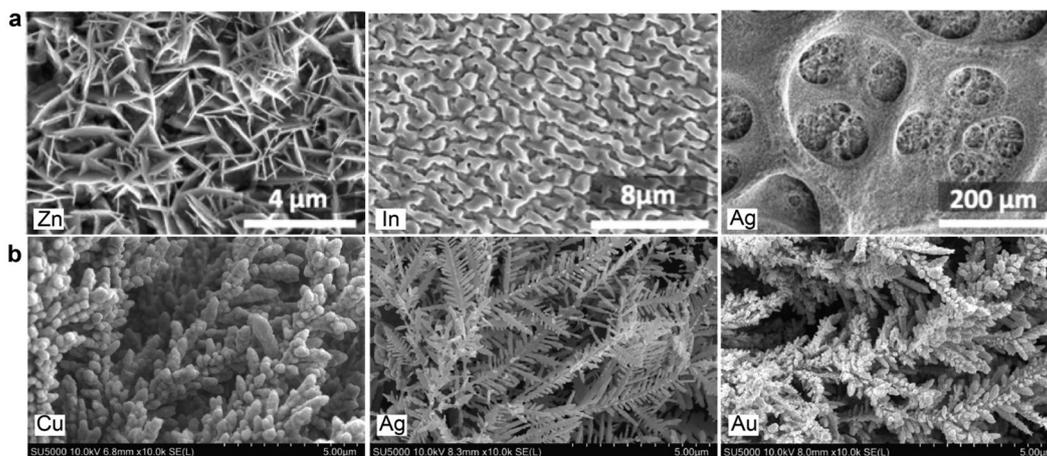
**Fig. 9** Scanning electron micrographs of (a) porous Zn, In, and Ag electrodes prepared by hydrogen-bubble-templated electrodeposition technique, reproduced with permission,<sup>60</sup> copyright 2017, John Wiley and Sons. (b) Cu, Ag, and Au nano dendrites on glassy carbon prepared *via* galvanic replacement reaction. Reproduced with permission,<sup>74</sup> copyright 2020, John Wiley and Sons.
