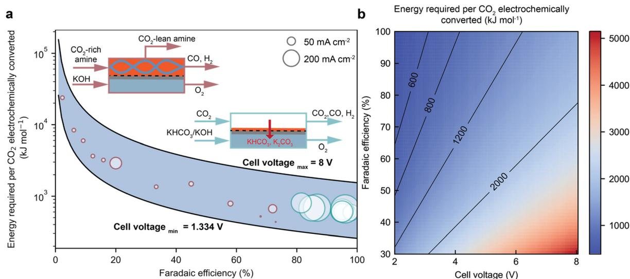
**Fig. 6** (a) A comparison of the energy consumption, CO faradaic efficiency, and cell potentials over integrated and gas-fed CO<sub>2</sub> electrolysis. (b) The role of CO faradaic efficiency and cell voltage in determining the overall energy consumption of CO<sub>2</sub> electrolysis to produce CO.<sup>36</sup>
