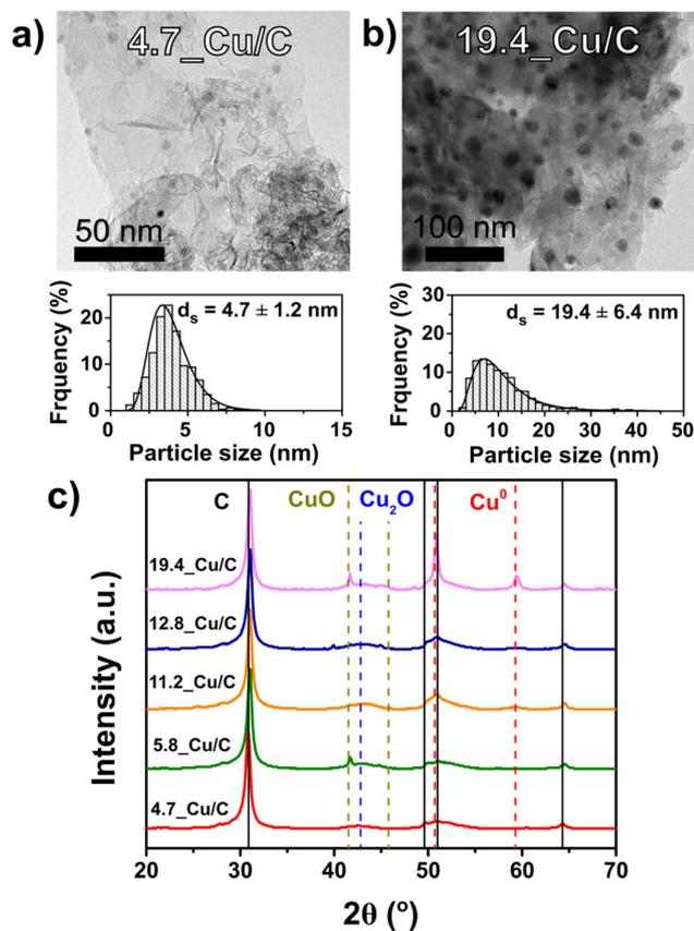
**Fig. 2** Transmission electron micrographs with corresponding particle size distributions of the 4.7\_Cu/C (a) and 19.4\_Cu/C (b) catalysts after activation. (c) Powder X-ray diffractograms of the activated Cu/C catalysts, diffractograms normalized to the intensity of the carbon (002) diffraction peak and vertically offset for clarity.
