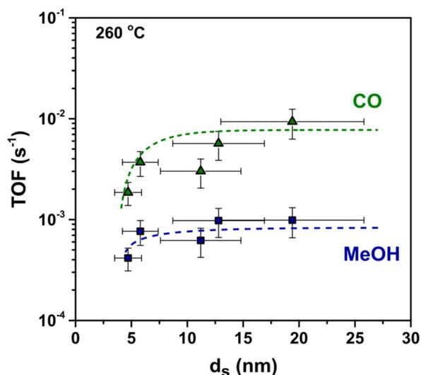
**Fig. 6** MeOH and CO TOF as a function of the Cu particle size. Trend lines were added to guide the eye. Reaction conditions: 4.2 mg of Cu per reactor, 40 bar(g), 260 °C, 600 mL min<sup>-1</sup> g<sub>Cu</sub><sup>-1</sup>, H<sub>2</sub>/CO<sub>2</sub>/He = 67.5/22.5/10 vol%.
