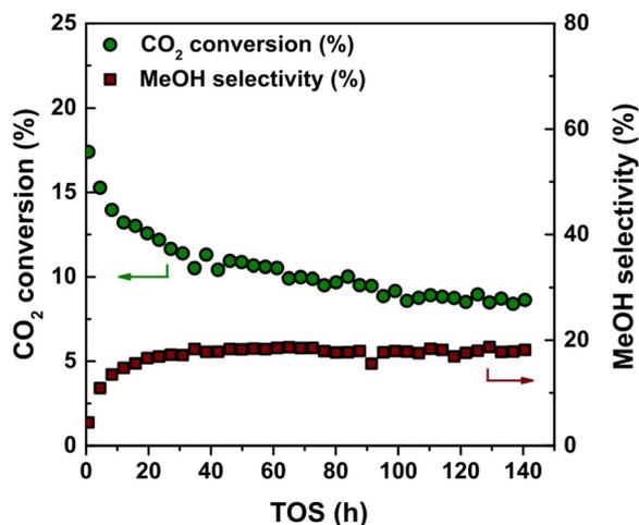
Fig. 1  $\text{CO}_2$  conversion and methanol selectivity as a function of time on stream (TOS) for the 4.7\_Cu/C catalyst with 5.2 wt% Cu. Reaction conditions: 4.2 mg of Cu per reactor, 40 bar(g), 260 °C,  $600 \text{ mL min}^{-1} \text{ g}_{\text{Cu}}^{-1}$ ,  $\text{H}_2/\text{CO}_2/\text{He} = 67.5/22.5/10 \text{ vol}\%$ .
