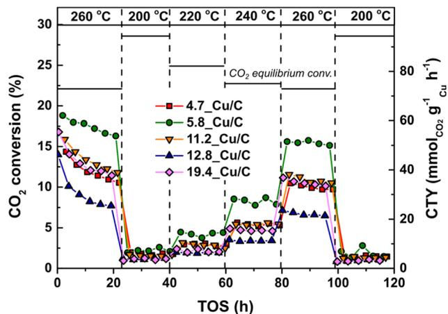
**Fig. 3** Characteristic profiles for CO<sub>2</sub> conversion and weight-normalized copper time yield for Cu/C catalysts as function of TOS (h) at different temperatures. Reaction conditions: 4.2 mg of Cu per reactor, 40 bar(g), 600 mL min<sup>-1</sup> g<sub>Cu</sub><sup>-1</sup>, H<sub>2</sub>/CO<sub>2</sub>/He = 67.5/22.5/10 vol%.
