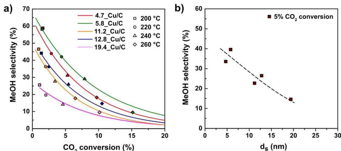
Fig. 5 (a) MeOH selectivity as a function of CO<sub>2</sub> conversion for catalysts with different Cu particle sizes. (b) Selectivity to MeOH as a function of Cu particle size for a CO<sub>2</sub> conversion of ~5%. The trend line was added to guide the eye. Reaction conditions: 4.2 mg of Cu per reactor, 40 bar(g), 600 mL min<sup>-1</sup> g<sub>Cu</sub><sup>-1</sup>, H<sub>2</sub>/CO<sub>2</sub>/He = 67.5/22.5/10 vol%.
