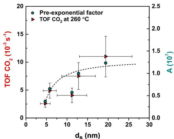
**Fig. 4** TOF and pre-exponential factor as a function of Cu particle size. Line is drawn to guide the eye. Reaction conditions: 4.2 mg of Cu per reactor, 40 bar(g), 260 °C, 600 mL min<sup>-1</sup> g<sub>Cu</sub><sup>-1</sup>, H<sub>2</sub>/CO<sub>2</sub>/He = 67.5/22.5/10 vol%.
