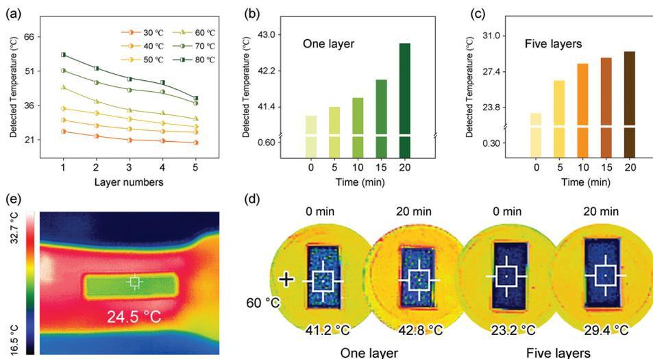
**Fig. 7** (a) Variation of the temperature detected on the upper surface of the NF@Co/C architecture with the number of layers at different heating temperatures. Variation of the temperature detected of (b) one-layer and (c) five-layer samples with heating time, as well as (d) the corresponding thermal infrared images. (e) Thermal infrared image of the NF@Co/C architecture placed on the arm.
