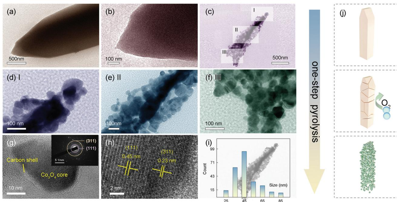
Fig. 3 TEM and HR-TEM images of (a), (b) ZIF-67, (c–h)  $\text{Co}_3\text{O}_4/\text{C}$ . Inset in (g) is the corresponding SAED pattern. (i) Size distribution of  $\text{Co}_3\text{O}_4/\text{C}$  nanoparticles. (j) Schematic illustration for the pyrolysis from ZIF-67 to  $\text{Co}_3\text{O}_4/\text{C}$ .
