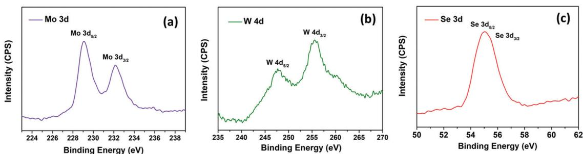
Fig. 4 XPS spectra of  $\text{MoSe}_2@WSe_2/CC$  (a) Mo 3d core level peaks region spectrum, (b) W 4d core level peaks region spectrum, (c) Se 3d core level peaks region spectrum.
