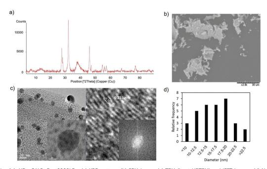
Fig. 5 Synthesis of AgNPs-CALB-Dext2000kDa. (a) XRD pattern. (b) SEM image. (c) TEM (inset HRTEM) and IFFT images. (d) Nanoparticle size distribution.
