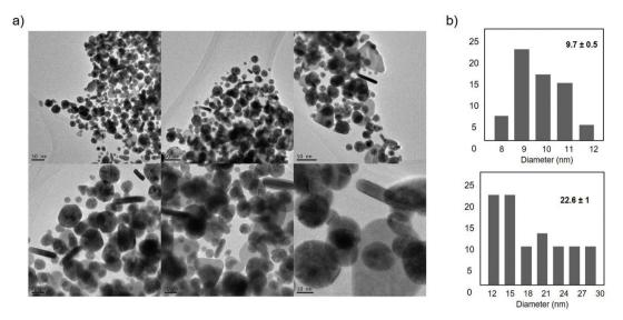
Fig. 10 Characterization of synthesized AuNPs-CALB-Dext6kDa hybrid. (a) TEM images. (b) Nanoparticles size distribution.
