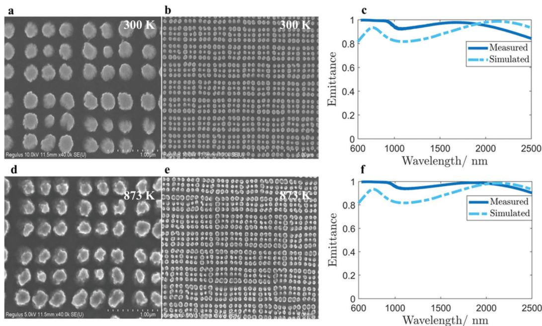
**Fig. 5** SEM images of the emitter and the measured emittance (a) at 300 K with a scale bar of 1 μm and (b) at 300 K with a scale bar of 5 μm. (c) Comparison of the measured and simulated emittances at 300 K, (d) at 873 K with a scale bar of 1 μm, and (e) at 873 K with a scale bar of 5 μm. (f) Comparison of the measured and simulated emittances at 873 K.
