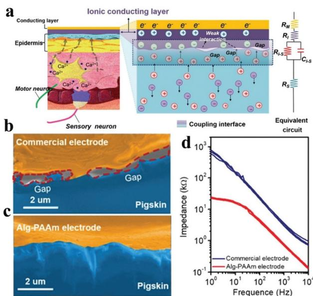
**Fig. 10** (a) Schematic of the electrode and skin used for EMG detection: describes the coupling process between ion flux (electrolyzed tissue medium) and current (electrode); SEM pictures display the interfacial clearance between pigskin and (b) commercial electrode or (c) Alg-PAAm electrode, respectively, (d) the impedance diagram of the electrode–skin system from 1–10<sup>4</sup> Hz. Reproduced with permission from ref. 51. Copyright 2020, Wiley-VCH.
