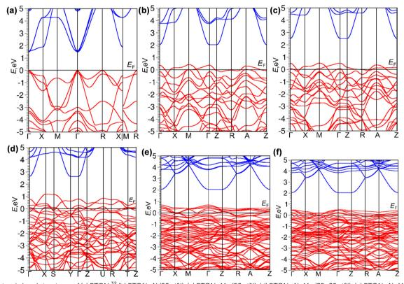
Fig. 5 Electronic band structures of (a) BTON: Al (50 at%), (c) BTON: Mg (50 at%), (d) BTON: Al: Mg (25: 25 at%), (e) BTON: Al: Mg (37.5: 12.5 at%), and (f) BTON: Al: Mg (12.5: 37.5 at%). The Fermi level is set at 0 eV.
