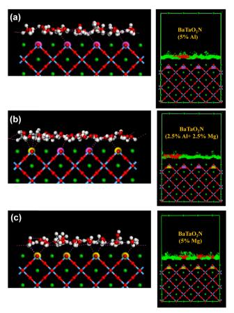
Fig. 7 Water and methanol molecules and field density distribution on the BaTaO<sub>2</sub>N(110) surfaces with 5% Al (a), 2.5% Al and 2.5% Mg (b), and 5% Mg (c). Atoms: grey - hydrogen, red - oxygen, blue - nitrogen, yellow magnesium, pink - aluminum, light blue - tantalum, green - barium; Isosurface: red - methanol, green - water.
