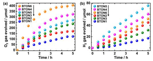
Fig. 6 Reaction time courses for photocatalytic O2 (a) and H2 (b) evolution over BTON1, BTON2, BTON3, BTON4, BTON5, and BTON6 loaded with CoO<sub>x</sub> and Pt nanoparticles as O<sub>2</sub> and H<sub>2</sub> evolution cocatalysts under visible light irradiation
