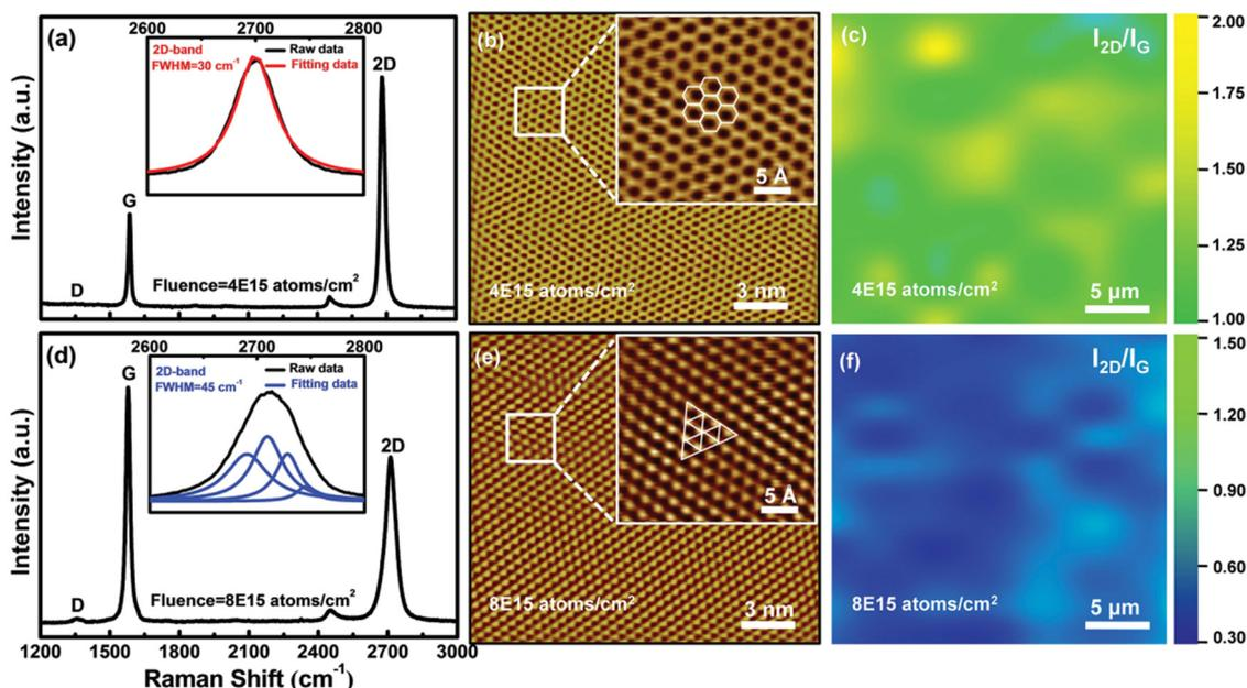
Fig. 8 Raman spectra of the (a) monolayer and (d) bilayer graphene. STM topographical images of the (b) monolayer and (e) bilayer graphene. The  $I_{2D}/I_G$  peak ratio derived from Raman mapping conducted on the (c) monolayer and (f) bilayer graphene. Reproduced with permission from ref. 53. Copyright 2015, Wiley-VCH.
