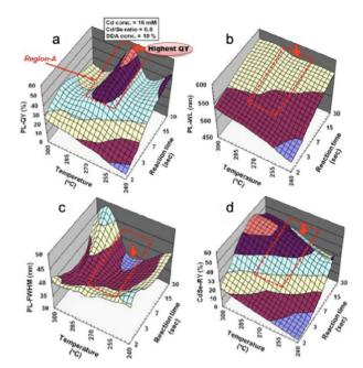
Fig. 5 A study of CdSe QDs by Orimoto et al. 107 An NN model of a 3D parameter space, where the output variables of (a) PLQY, (b) PL wavelength (nm), (c) FWHM (nm), and (d) reaction yield (RY, %), varying as a function of temperature (°C) and reaction time (s). The red arrow indicates the point corresponding to the highest PLQY. Reprinted with permission from ref. 107. Copyright 2021 American Chemical Society.
