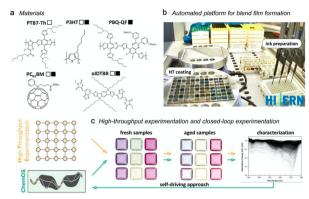
Fig. 11 A study of organic photovoltaic (OPV) thin films by Langner et  $\it{al}.^{132}$  (a) The three polymer donors and the two small molecule acceptors studied, where the open and closed squares indicate the two sets of four that were studied. (b) The automated system for ink formulation, deposition, film formation and characterization, (c) The process workflow showing the two approaches used (HTE grid-based versus ML-guided). Reprinted with permission from ref. 132.
