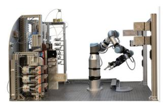
Fig. 9 A study by Coley et al. 130, where an Al-driven automated flow chemistry system using a microfluidic reactor platform was embedded in a larger system, including a robot arm for configuring the system between each run. From ref. 130. Reprinted with permission from AAAS.
