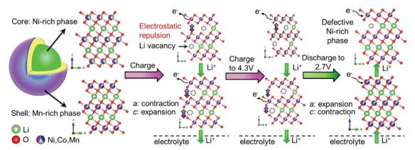
Fig. 9 Schematic illustration of a subsequent (de)lithiation mechanism in the core-shell NCM cathode materials during the first cycle, showing an obvious change in the unit-cell volume of the Ni-rich phase within the interior region of a secondary particle with respect to the Mn-rich phase. TM: Ni whitish; Mn - magenta; Co - blue. Reproduced from ref. 179 with permission from the Authors, Elsevier Ltd.
