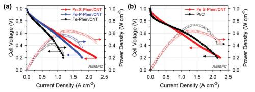
Fig. 5 Alkaline AEMFC performance of MEAs using (a) Fe-Phen/CNT, Fe-P-Phen/CNT, and Fe-S-Phen/CNT as cathode catalysts and (b) Fe-S-Phen/CNT and Pt/C as cathode catalysts. Reproduced from ref. 76 with permission from the American Chemical Society.
