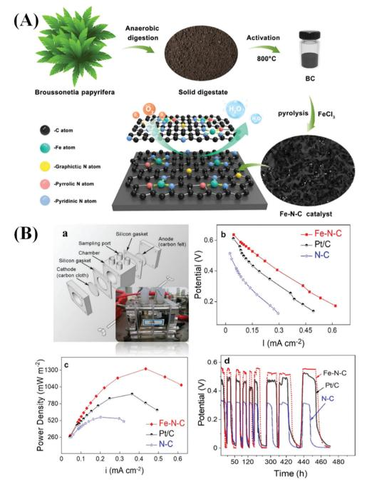
Fig. 7 (A) Schematic illustration of the fabrication of hierarchical Fe-N-C catalysts derived from the solid digestate. (B) Schematic illustration of a singlechamber MFC (a); power density (b) and electrode polarization curves (c), and the periodic variation of single-chamber MFCs coupled with the Fe-N-C, Pt/C, and N-C catalysts (d). Reproduced from ref. 133 with permission from the American Chemical Society
