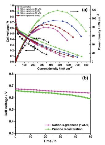
Fig. 6 (a) DMFC performance of pristine Nafion and Nafion-S-graphene hybrid membrane at 70 °C under ambient pressure. (b) Stability test of the membranes for 50 h under fuel cell configuration at OCV. Reproduced from ref. 121 with permission from the American Chemical Society.
