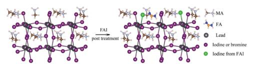
Fig. 6 Schematic illustration of the filling of I<sup>-</sup> and MA<sup>+</sup> vacancies in the perovskite films by the FAI post-treatment process<sup>133</sup> [Reprinted with permission. Copyright (2018) American Chemical Society].
