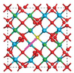
Fig. 4 General schematic of the formation path of a Frenkel pair defect (highlighted in pink) in  $La_2Hf_2O_7^{70}$  [Reprinted with permission. Copyright (2017) American Chemical Society)
