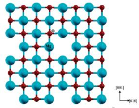
Fig. 5 Schematic representation of a Schottky defect<sup>71</sup> [Reprinted with permission. Copyright (2004) American Chemical Society].
