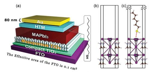
Fig. 2 A schematic representation of a typical perovskite-based photovoltaic cell<sup>67</sup> [Reprinted with permission. Copyright (2018) American Chemical Society].
