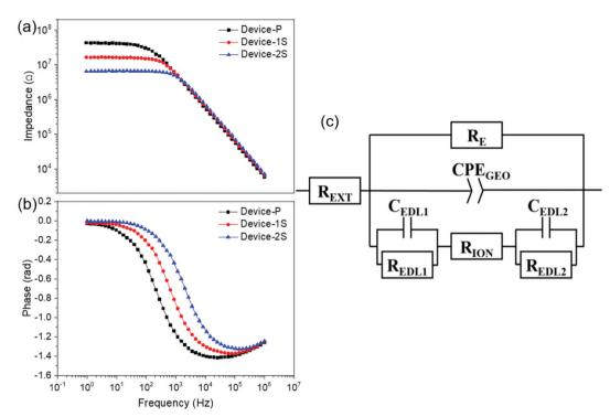
Fig. 2 ElS curves of  $Ru(bpy)_3(PF_6)_2$  memristor devices with different concentrations of  $LiClO_4$ . (a) Impedance *versus* frequency data and (b) phase *versus* frequency data for Device-P (black squares), Device-1S (red circles), and Device-2S (blue triangles). (c) An equivalent circuit employed for ElS fitting of the OMIEC memristor devices.
