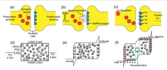
Fig. 1 Schematic illustration of the mechanisms of a biological synapse (a-c) and an OMIEC memristor (d-f).
