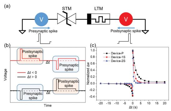
Fig. 7 (a) A series circuit for the STDP simulation, (b) presynaptic and postsynaptic spikes, applied pulse on a series circuit; short pulse: 14 V (pre) and 18 V (post) with 500  $\mu$ s, long pulse: 6 V with 200 ms,  $\Delta t$ : 50 ms-20 s, and (c) normalized weight change versus time difference for OMIEC devices.
