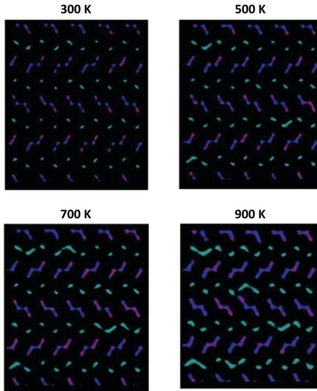
Fig. 8 Comparison among the  $\text{Na}^+$  ion trajectories of  $\text{Na}_{0.44}\text{MnO}_2$  sample, with 71% of Na1 sites occupied, as the temperature changes: view along the  $c$  axis (see Fig. S4, ESI† – for a view along the  $a$  axis). For the sake of clarity, only the positions occupied by the  $\text{Na}^+$  ions are reported; each point represents a position occupied by  $\text{Na}^+$  along the simulation time. Legend: Na1 – cyan; Na2 – purple; Na3 – blue.
