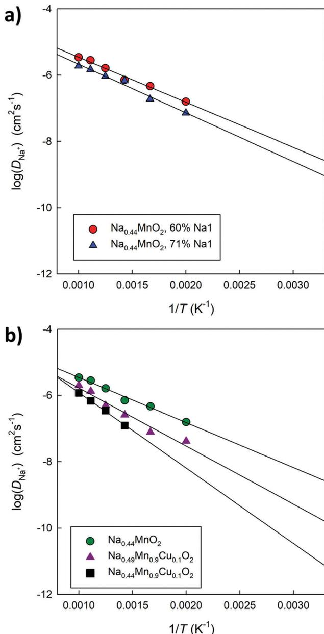
**Fig. 12** Arrhenius plot of  $\text{Na}^+$  diffusion coefficients ( $D$ ) for (a) two different models having the same composition ( $\text{Na}_{0.44}\text{MnO}_2$ ) and characterized by a different distribution of  $\text{Na}^+$  ions between 1D and 2D channels; and (b) three different models having the same occupation of the Na1 site (60%) but different composition.
