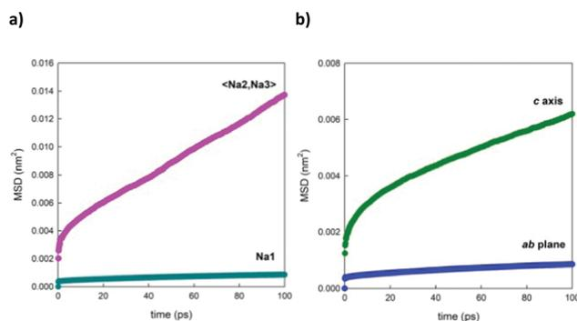
Fig. 11 Comparison between the MSD vs. time plots of Na<sup>+</sup> ions (a) positioned in 1D channels (Na1) and 2D channels (averaged over Na2 and Na3) and (b) diffusing along the *c* axis or in the *ab* plane (averaged over all the Na<sup>+</sup> ions in the simulation box). As a selected example, the data related to Na<sub>0.44</sub>MnO<sub>2</sub> (71% of Na1 occupation) at a simulation temperature of 500 K are reported.
