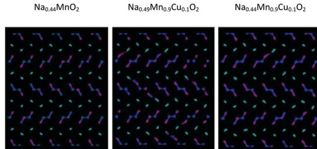
Fig. 10 Comparison among the Na<sup>+</sup> ion trajectories at 700 K for a given occupation of the Na1 crystallographic sites (60%) as the composition changes: view along the *c* axis.
