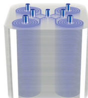
Fig. 1 Development of a mass-producible and deformation-free plastic spiral inertial microfluidic device. (a) A schematic diagram representing the fabrication process of the conventional polydimethylsiloxane (PDMS) spiral device and its stacking process for high-throughput application. (b) A schematic diagram representing the channel deformation in the PDMS spiral device and its effects on the device operation and performance; the color represents the relative channel deformation. (c) A schematic diagram representing the fabrication process of the plastic device and its key advantages; the plastic spiral device was designed by compensating for the channel deformation in the PDMS spiral device.
