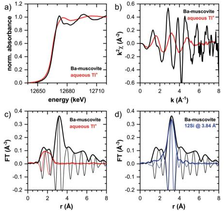
Fig. 3 XANES and EXAFS reference spectra of Tl-rich Ba-muscovite and of 10 mM aqueous Tl<sup>+</sup>: (a) XANES spectra, (b)  $k^2$ -weighted EXAFS spectra, (c) Fourier-transform of  $k^2$ -weighted EXAFS spectra (magnitudes: thick lines; imaginary parts: thin lines). (d) Fourier-transform of EXAFS spectrum of Tl-rich Ba-muscovite compared with shell-fit involving 12 Si atoms at a distance of 3.84 Å from Tl.
