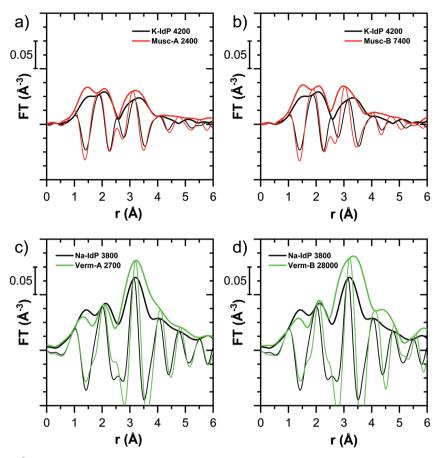
Fig. 7 Fourier-transformed  $k^2$ -weighted Tl  $L_{III}$ -edge EXAFS spectra of (a and b) Tl-loaded muscovites Musc-A and Musc-B compared to Tlloaded K-IdP and of (c and d) Tl-loaded vermiculites Verm-A and Verm-B compared to Tl-loaded Na-IdP. Numbers in sample names indicate the Tl loading of the phyllosilicates in  $mg kg^{-1}$ .
