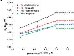
Fig. 8 Determination of the diffusion coefficient (A) and the charge transfer coefficient (B) from extracted data of the cyclic voltammograms. Reproduced with permission from N. Kostevšek, K. Ž. Rožman, D. Pečko, B. Pihlar and S. Kobe, Electrochim. Acta, 2014, 125, 320.63
