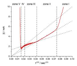
Fig. 7 Current of the electrodeposition of copper into 30  $\mu$ m thick TEPC membranes with 400 to 450 nm nanopores plotted against  $t^{-0.5}$ . The electrolyte for the deposition contained 0.25 mol  $L^{-1}$  CuSO<sub>4</sub>·5H<sub>2</sub>O and 2 mol  $L^{-1}$   $H_2SO_4$ . Reproduced with permission from I. U. Schuchert, M. E. T. Molares, D. Dobrev, J. Vetter, R. Neumann and M. Martin, J. Electrochem. Soc., 2003, 150, C189.58
