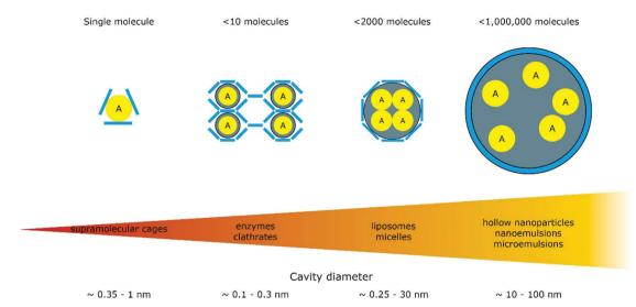
Fig. 21 Schematic description of the different types of single entity colloidal confinement discussed within this work. An increasing cavity size and accessibility by means of electrochemical methods is indicated by an increasing arrow size. The yellow spheres tagged with "A" symbolize single encapsulated molecules, the blue-grey spheres symbolize the presence of solvent molecules within the cavitand, the light blue objects describe parts of the cavitand
