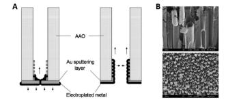
Fig. 6 (A) Influence of the contact sputtering process of a blocked and unblocked membrane onto the seed formation and the following electrodeposition of nanomaterials. (B) SEM images of the resulting CoPt nanotubes and nanowires. Reproduced with permission from J. Fu, S. Cherevko and C.-H. Chung, Electrochem. Commun., 2008, 10, 514.5
