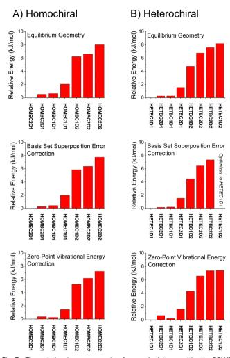
Fig. 7 The relative isomer energies from calculations with the B3LYP GD3BJ def2TVP model chemistry are shown with three different levels of approximation. The top set of results uses the equilibrium energies. The middle panel includes a counterpoise correction to account for basis set superposition error. The bottom panel uses equilibrium energies correct by the zero-point vibrational energy contribution using the harmonic approximation.
