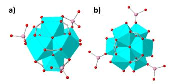
Fig. 4 The coordination mode of (a) As(v) and (b) As(iii) species (Arsenic atoms shown as pink balls) in the structures of **HEX-MOF/As(vi)** and **HEX-MOF/As(iii)** respectively, as determined *via* Rietveld refinement.
