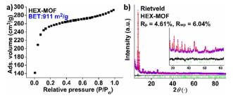
Fig. 1 (a) N<sub>2</sub> sorption isotherm (77 K) for HEX-MOF. (b) Rietveld plot of HEX-MOF. Violet crosses: experimental points; red line: calculated pattern; black line: difference pattern (exp-calc); and green bars: Bragg positions. Inset: Magnification of the  $2\theta$  region  $30-60^{\circ}$ .
