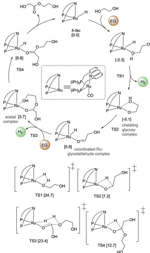
Fig. 26 Mechanism of EG dehydrogenative coupling. Calculated free energies are in kcal mol<sup>-1</sup> with respect to **4-fac** + 2\*EG.
