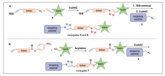
Scheme 1 Synthetic approach towards a modular assembly of conjugates 5, 6, and 7 employing linkers with suitable orthogonal protecting groups; (A) PEG-linked and disulfide-containing bio-reducible conjugate 5 and 6 of amatoxin 4; (B) Cathepsin B cleavable self-immolative conjugate of amatoxin 3.
