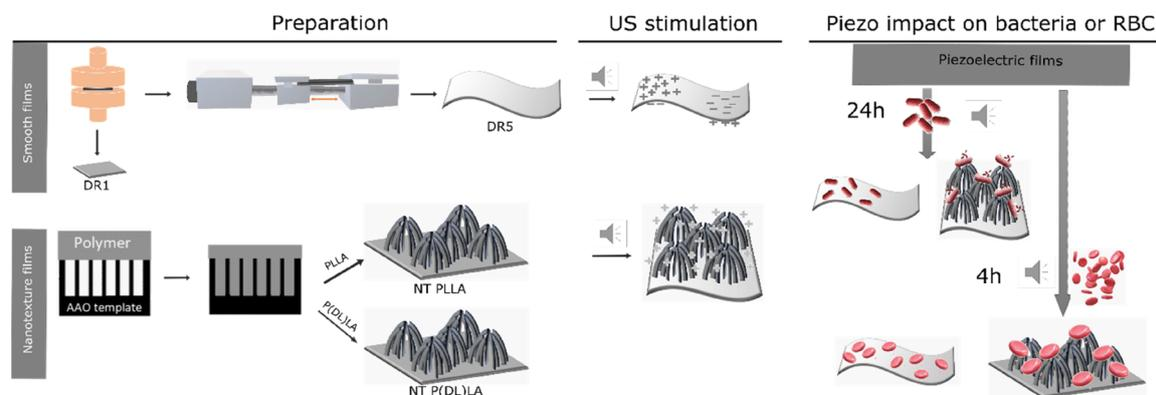
**Fig. 1** Schematic presentation of the preparation of smooth piezoelectric (DR5) and non-piezoelectric (DR1) and nanotextured piezoelectric (NT PLLA) and non-piezoelectric (NT P(DL)LA) polymer films and their expected response to ultrasound stimuli as generation of positive charge on the stretched upper side of the down bent polymer and negative charge on the bottom bent side; and piezo-stimulated damaging impact on bacteria for nanotextured film and not harmful behaviour towards RBCs.
