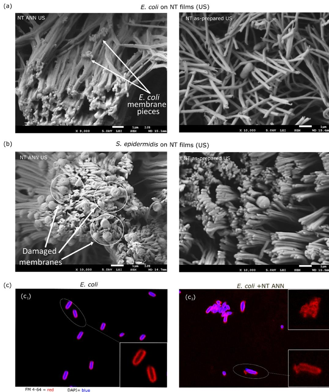
**Fig. 9** SEM images of (a) *E. coli* and (b) *S. epidermidis* bacteria on the nanotextured film surfaces after US stimulation for 30 min following 24 h incubation in saline suspension after cell fixation for NT ANN sample (left) and NT as-prepared sample. (c) FM 4-64 (red) and DAPI (blue) staining of *E. coli* bacteria (c<sub>1</sub>) and bacteria in contact with NT ANN film (c<sub>2</sub>) after test in saline solution with US stimulation.
