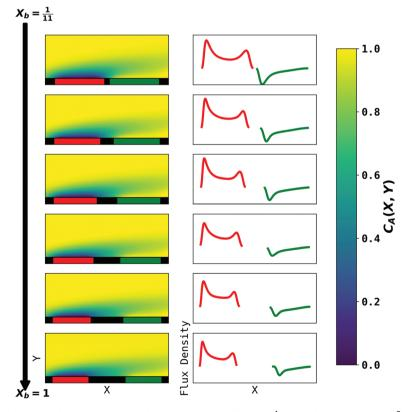
Fig. 6 PINN prediction of double channel electrode at steady state by varying  $X_b$  from  $\frac{1}{11}$  to 1 with a step size of  $\frac{2}{11}$  while the length of generator and detector electrode are equal. (left) Concentration profile at steady state. Generator electrode, detector electrode and insulating material are represented with red, green and black boxes. (right) Flux density at each electrode. Red line and blue line are for generator and detector electrode respectively.
