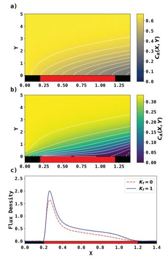
Fig. 8 PINN prediction of channel electrode coupled with CE reaction, when  $K_{\rm f}=1$ ,  $K_{\rm eq}=0.5$  and Pe = 1.59. (a and b) Concentration profile of R and A respectively. (c) Flux density of electrochemical reaction of A when  $K_{\rm f}=0$  and  $K_{\rm f}=1$ .
