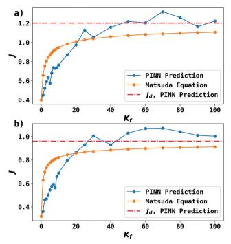
**Fig. 9** PINN prediction of kinetic flux (orange line with marker) as a function of dimensionless forward reaction rate constant at fixed  $K_{\rm eq}$  and comparison with flux predicting by Matsuda equation (blue line with marker). Red dash-dot line represents the mass transport limiting current when  $C_{\rm A}^*=1$ . (a)  $K_{\rm eq}=0.5$ , Pe = 6.38, (b)  $K_{\rm eq}=0.5$ , Pe = 1.59.
