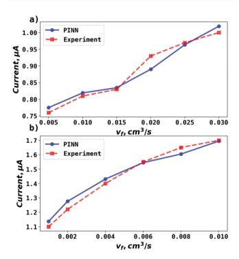
Fig. 5 Compare PINN prediction with experiment for oxidation of ferrocene at different electrode length. (a) Electrode length,  $x_{\rm e}=4~\mu m$ . (b) Electrode length,  $x_{\rm e}=11~\mu m$ .
