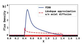
Fig. 3 PINN prediction of transport-limited current at microband electrode when Pe = 2.9. (a) Concentration profile at steady state. (b) Flux density at steady state for the channel electrode using PINN without simplification (blue line); flux density predicted by PINN using Lévêque approximation and neglecting axial diffusion (red dashed-line). Red square represents the electrode and black squares are the insulating material.
