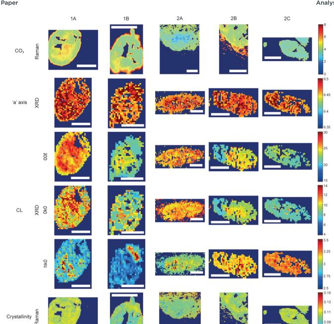
Fig. 4 Hydroxyapatite feature patterns across calcifications. Maps of calcifications for total carbonate content (%) measured using Raman; length of the unit cell 'a' axis (nm) and coherence length (nm) measured using XRD; and crystallinity (cm) measured with Raman using 1/FWHM of the phosphate peak at 960 cm $^{-1}$ . Scale bars = 150  $\mu$ m.
