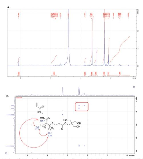
Fig. 2 The NMR analysis for 1:1 (thiol:ene) gel after basic degradation with sodium hydroxide in deuterium oxide solvent (D<sub>2</sub>O, 400 MHz): (A) the <sup>1</sup>H NMR spectrum of the hydrolysis product; (B) the gHMBC spectrum for the hydrolysis product with key correlations highlighted.
