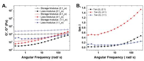
Fig. 4 (A) Comparative storage and loss moduli for representative samples from each gel composition of MBA and PTK with respect to thiol:ene functionality from frequency sweep measurements; (B) plot of  $\tan (\delta)$  as a function of angular frequency
