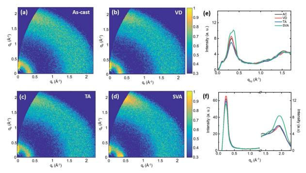
Fig. 3 GIWAXS 2-D images (a-d) and their corresponding in-plane (e) and out-of-plane (f) line cuts.
