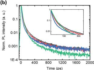
Fig. 5 Steady-state (a) and time-resolved (b) photoluminescence (PL) of the IT-4F film and TPD-3F:IT-4F solar cells excited at 400 nm. The time resolved traces are integrated over the whole spectra.
