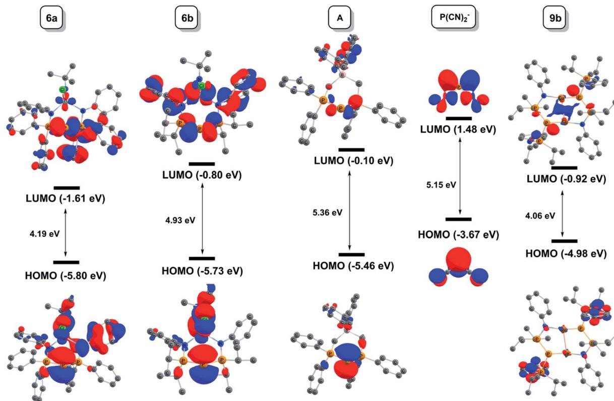
Fig. 4 HOMO and LUMO for complexes 6a, 6b, A, P(CN)<sub>2</sub><sup>-</sup> and 9b (cut-off 0.05).
