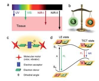
Fig. 2 (a) Schematic tissue penetration depth of light with different wavelengths. (b) The balance between emission wavelength ( $\lambda$ ) and efficiency ( $\Phi$ ). (c) The molecular design strategy of NIR-II AlEgens. (d) Jablonski diagrams of TICT dynamics.
