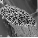
Fig. 1 SEM micrographs showing the change in the size of the microchannels before and after the modification. (a) Natural henequen fiber (b) henequen fiber modified with copper phthalocyanine
