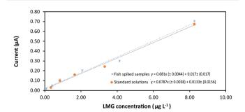
Fig. 6 Calibration plot of LMG. Comparison of the analytical sensitivity (slope) using standard solutions and fish spiked samples. Linear interval  $0.082-8.262~\mu g~kg^{-1}$ .
