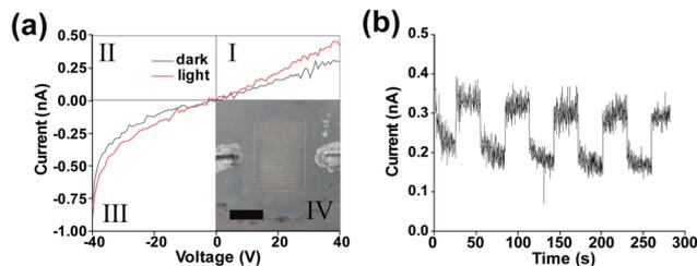
Fig. 2 (a) IV curves of printed contacts SnS device under darkness and AM1.5 illumination with inset photograph of pseudo Langmuir-Blodgett device with printed Ag contacts scale bar 5  $\mu\text{m}$ . (b) Device under +40 V bias under fixed darkness/illumination cycle.
