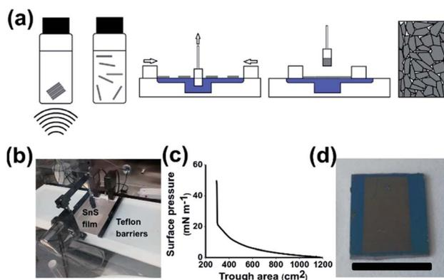
Scheme 1 Preparation of SnS nanosheet thin films *via* the Langmuir–Blodgett method. (a) Cartoon of Langmuir–Blodgett film preparation. (b) Image of Langmuir–Blodgett trough with compressed SnS film. (c) Surface pressure profile during film compression. (d) Image of sample prepared on Si/SiO<sub>2</sub> substrate with edges masked (scale bar 1.5 cm).
