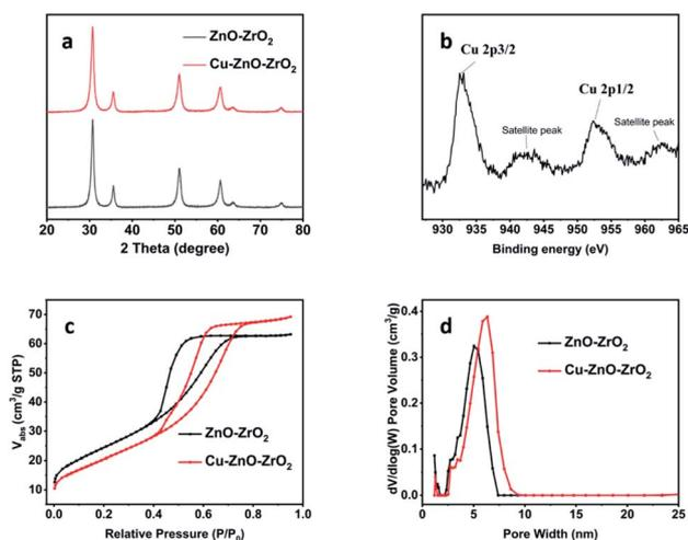
Fig. 1 PXRD patterns (a), high-resolution XPS of Cu element (b), nitrogen isotherms (c), and pore size distribution (d) for the catalyst Cu–ZnO–ZrO<sub>2</sub> and the pristine bimetal oxide support ZnO–ZrO<sub>2</sub>.
