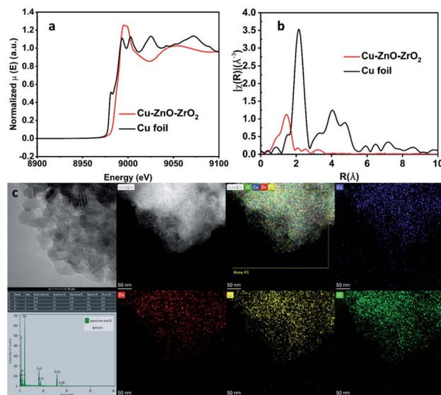
Fig. 2 Characterizations of the catalyst Cu–ZnO–ZrO<sub>2</sub>. XANES (a), EXAFS (b), and AC-HAADF (c) with EDS mapping. Cu (blue), Zn (red), Zr (yellow), and O (green).
