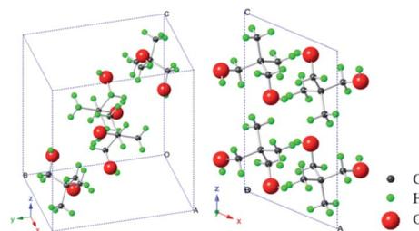
**Scheme 1** Crystal structure (monoclinic phase) of NPG at 295 K.<sup>15</sup> Notes: left, view along (1 1 1) crystal plane; right, view along (0 1 0) crystal plane.
