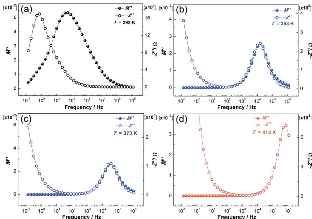
Fig. 7 The temperature dependence of  $M''$  (the imaginary part of complex electric modulus) and  $-Z''$  (the imaginary part of the complex impedance) at selected temperatures of 293 K (a), 353 K (b), 373 K (c) and 413 K (d).
