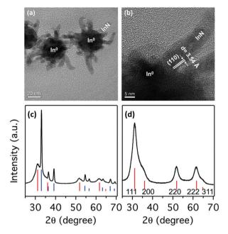
Fig. 22 TEM images of the NPs. (a) Overview of the as prepared sample, showing the InN branches stemming out of larger In(0) NPs. (b) HRTEM image of one of the InN branches in (a) at the surface of the In (0) nanoparticle. XRD pattern for the (c) as-prepared sample and (d) acid treated sample. The vertical lines show the XRD patterns of bulk zinc blende-InN (red) and tetragonal In(0) (blue). Reprinted with permission from ref. 176. Copyright 2016 American Chemical Society.
